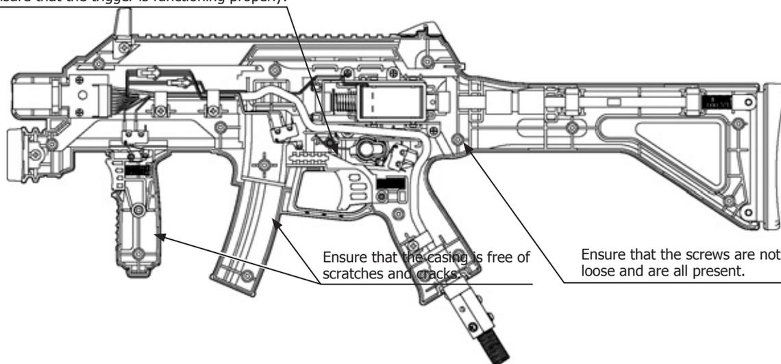
Ensure that the casing is free of scratches and cracks.
