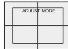
Make adjustment so as to have red superimposed on green. When red is superimposed on green, the color becomes yellow.
