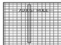
The selected column line or row line (shown left is the column line) can be moved in the desired up/down or right/left directions as applicable.
