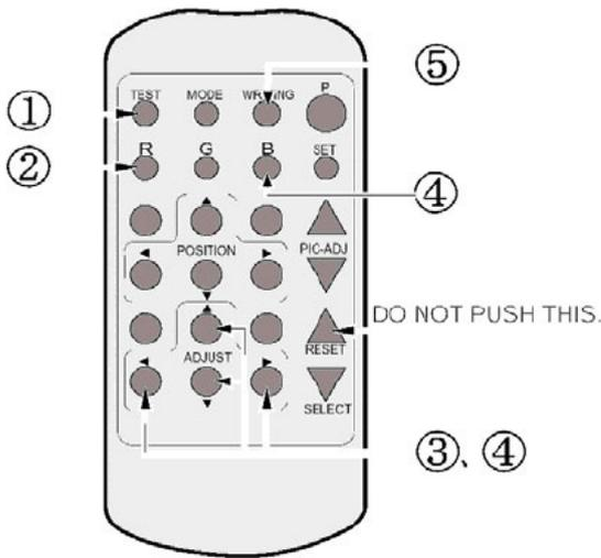
When either of ② ④ COLOR SELECT buttons (R, B) is pressed, if the color desired to be adjusted disappears, press that particular button again. For example, if the red color needs to be adjusted again at the stage of ④, the R button need to be pressed twice.
