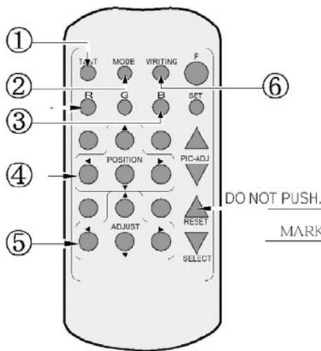
(Note 1) When the MODE button is repeatedly pressed, the adjustment modes will circulate as follows:
