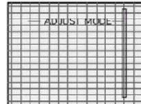
Use the ◀ ▶ buttons to select the column line, and the MARKER moves in the right/left direction. However, the movable range is predetermined.
