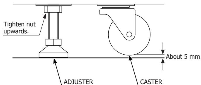
FIG. 6-2c Aligning the Adjusters
