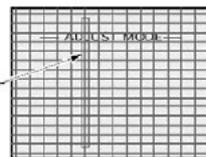
The crosshatch test pattern appears and the vertically long MARKER is shown.
