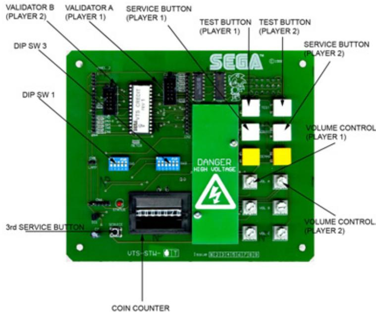
FIG. 9-1a VTS Board
