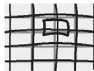
Although the direct vicinity of the MARKER's center moves most conspicuously, make adjustment by paying attention to the periphery area also. Shown left is the magnified MARKER periphery.
